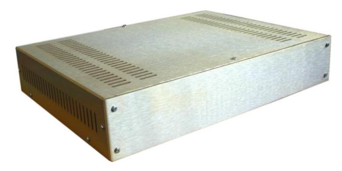
A newly added **STANDARD ENCLOSURES** 20 Series provides an off the shelf and economical way to package the table-top instrument and HI-FI equipment. This series is made from .09" thick aluminum base to handle the heavy components. To achieve this high quality appearance, we include the .12" thick front panel and painted top cover with texture finish in either black or gray.
